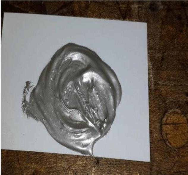
9. Mix the epoxy thoroughly for 45 seconds. There is a 2 minute work time once the epoxy is mixed.
