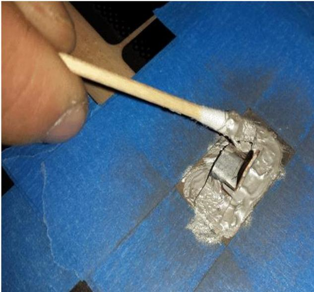
10. Apply the epoxy to completely cover the terminal foot/feet and the prepared area of the defroster grid. Smooth out the epoxy for a good contact between the terminal and defroster grid within the two minute work time.
