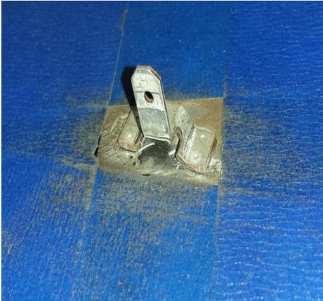
7. Press the terminal onto the defroster grid and hold for 1 minute. After releasing allow 5 minutes to form a secure bond.
